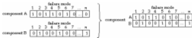
Figure 2. Forming a component-failure matrix.
