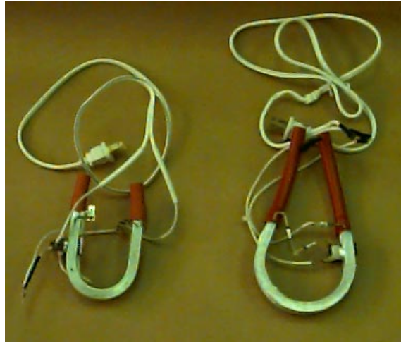
Figure 5: The convert electricity to thermal energy module for the Brand A tea brewer and the Brand A coffee maker.
