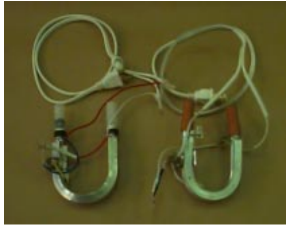
Figure 2: The convert electricity to thermal energy module for both tea brewers.
